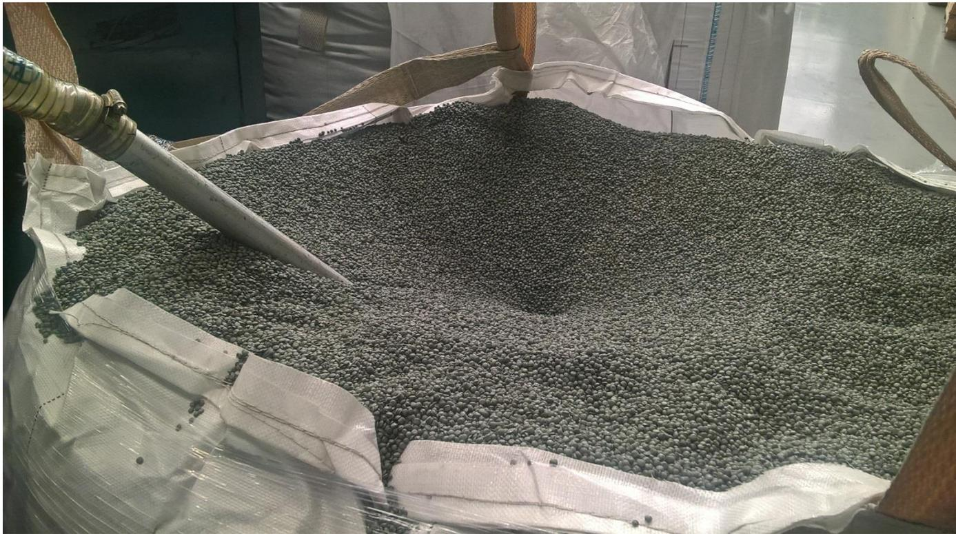
**Astron 3 --- The pellets of waste plastic are extruded into sheets of Tuffboard.**
